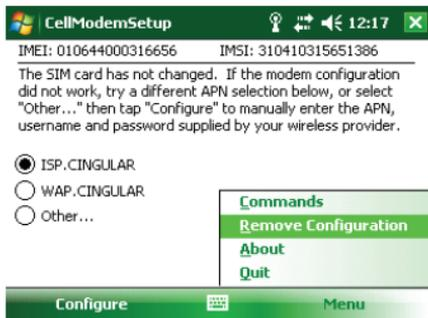
2. The modem configurations are removed from the handheld. During the process the handheld performs a reset to complete this process
