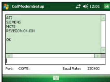
The current port is displayed along with the current baud rate. In this example, the GSM modem has not yet been configured. Port: is "COM5." When it is configured, Port: will be "VCA1."
