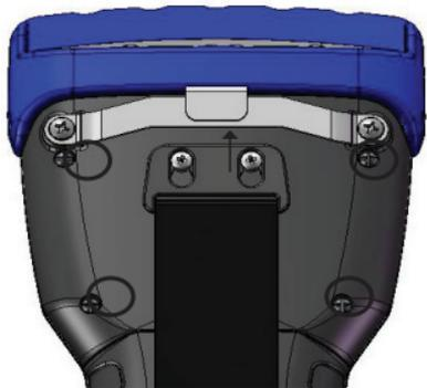
4. Slide the top of the hand strap up to detach it from the back. Remove the bottom of the hand strap. (The hand strap is not used with the pack. Place the hand strap someplace where you can find it in the future.)
