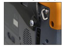
4. Press the back of the handle firmly against the tablet and align the left screw hole.
