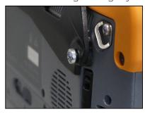
4. Press the back of the handle firmly against the tablet and align the left screw hole.
