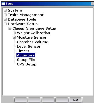
Figure 3-21: Select Actuators from the Setup menu to access the Actuator Setup screen
