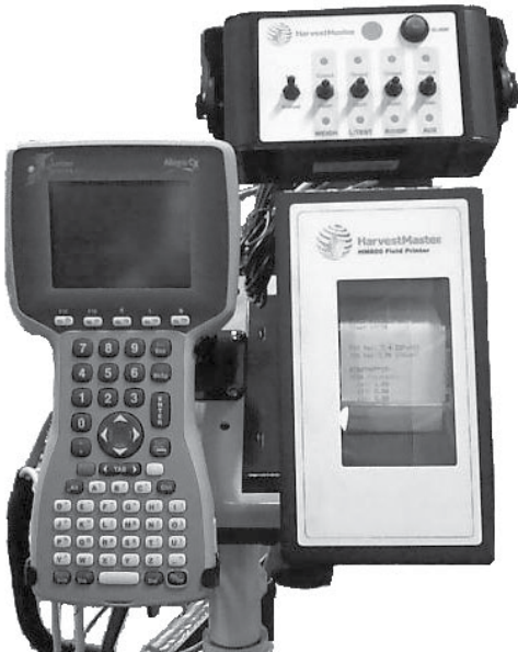
Figure C-1: Front view of HM-800 components
