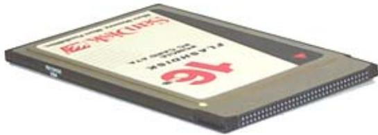
The PC card slot accepts Type I or Type II cards. These cards include ATA Flash cards, SRAM (Static Random Access Memory), and Compact Flash adapter cards. All types of cards have a 68 pin connector for attachment to the Allegro. The cards must be 5 V or 5 V/3 V (PC cards that are 3 V only are not supported). This is a 16 bit card slot. It is not a “card bus” slot.
