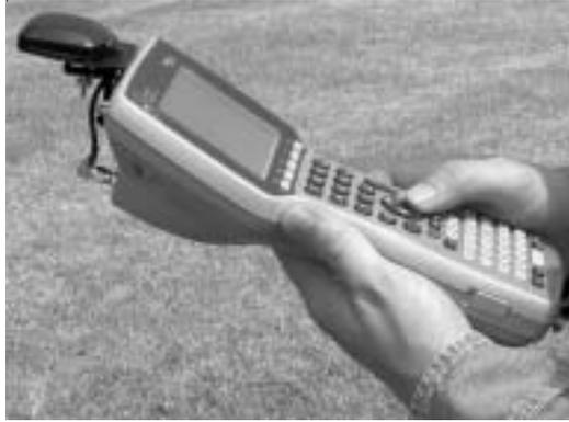
The Lassen LP module is a high-performance, low power, micro GPS receiver that supports both TSIP and NMEA protocols with autonomous accuracy of 5 –10 meters, or 2 – 5 meters after differential correction. The GPS expansion pod is used in conjunction with the following programs:
