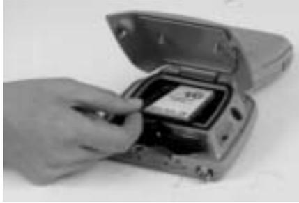
❖ *Important Note: Be careful when inserting and removing cards. Excess force could damage the card and the card drive. If the system tray indicator for the PC card activity is on, the computer is writing to the card. Do not turn off the Allegro and remove the card until the indicator stops blinking. Incomplete files can corrupt the data already stored on the card.*
