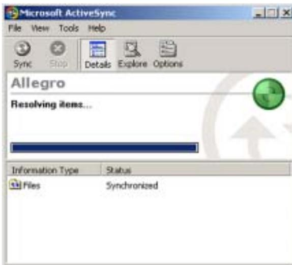
The file you select to be synchronized now replaces the existing file with the file chosen as the master file. In this example, the left arrow is selected and the file on the Allegro is transferred to the desktop PC, replacing the file on the desktop PC with the master file on the Allegro.
