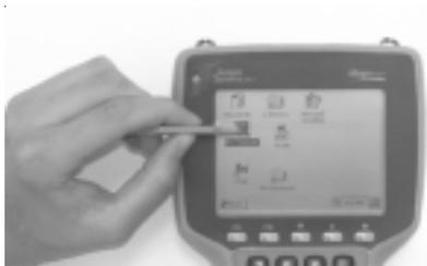
Three styli are provided: two small on-board stylus and a full size pen-type stylus. The small on-board stylus snaps into a holding bay built into the top of the Allegro. The Allegro can only hold one on-board stylus at a time. Other pointed objects can be used, including your finger. Be sure to use a device that will not scratch the screen.
