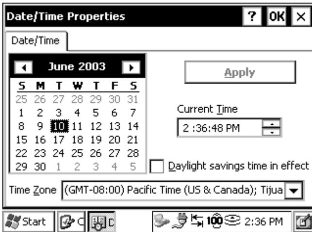
❖ *Note: The “Daylight savings time in effect” option does not affect the Current Time when this option is selected/deselected and applied. If you are in a time zone that is affected by daylight savings, select the “Daylight saving comes into effect on your calendar, the time automatically changes. Your Allegro receives a pop-up notification that your clock has changed.*
