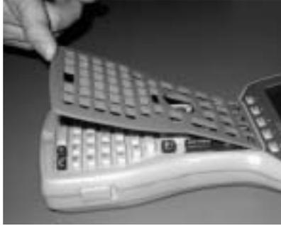
Reattach the bezel by carefully inserting the top ridge under the function keys and lowering the bezel down flat onto the case. Press down along the sides while aligning the keys through the holes.
