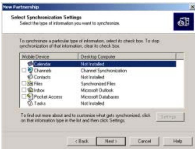
The *Synchronized Files* option is the only synchronization function currently operational with the Allegro. Additional options are not available.
