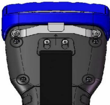
3. Remove the cover and screws from the handheld. (The cover is not used with the pack.
