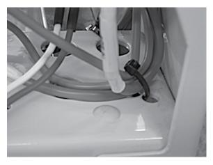
Figure D-9: Cables secured to frame with tie
