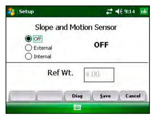
Figure 3-13: Enter the reference weight in the Slope & Motion Setup screen or select internal for HM800 system
