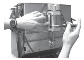
Figure 9-4: Loosening the limit switch
