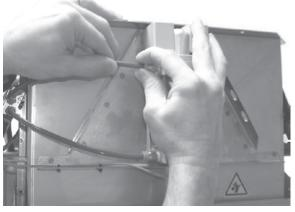
Figure 9-3: Removing the air hose
