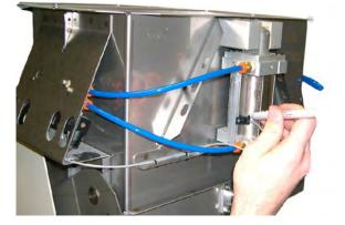
*Figure 9-12: Use a marker to make the top edge of the limit switch*
