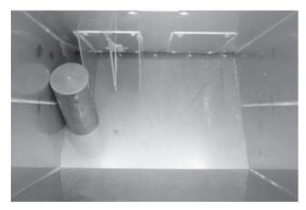
*Figure 3-5: Place the weight on the far side of the weigh bucket*
