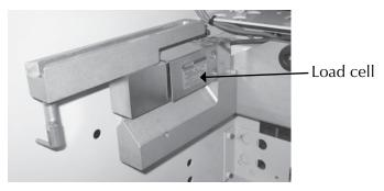
Figure 9-18: Load cell
