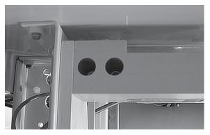
Figure 9-19: Bottom two screws of load cell
