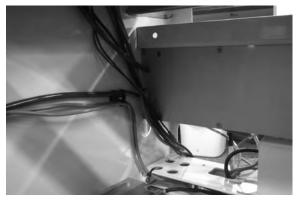
Figure D-8: Cables running down inside HCGG towards the modules
