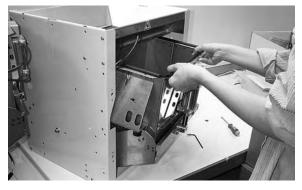
Figure 9-17: Removing the weigh bucket
