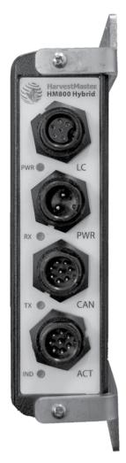
*Figure 4-3: Side view of BDS Hybrid showing connectors and labels.*
