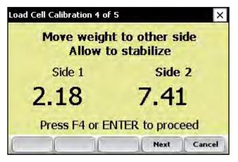
Figure 3-7: Load Cell Calibration screen 4 of 5
