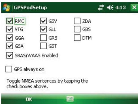
These settings work for most applications. To make changes to the default settings, exit all GPS programs on your Field PC (this is a requirement) and go to *Start > Programs > AMXU Pod Setup*.
