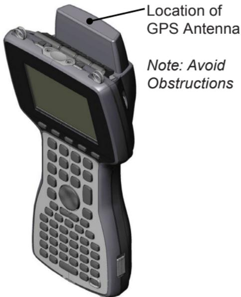
This integrated system includes a GPS Expansion Pod and GPS Pod Setup utility installed on a Field PC. Retrofits on existing Field PCs must be performed at the factory.
