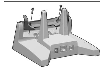
4. Provide power to the dock using the AC power cord and adapter. Plug the power cord into an AC power supply and the power adapter into the power input jack on the dock.
