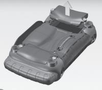
Loosen guarter turn latches to open battery compartment door.
