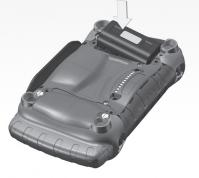
Place battery pack into the compartment.
