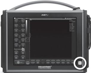
CHARGE THE 4VETJ INTERNAL BATTERY USING THE AC POWER SUPPLY FOR 4-6 HOURS 2 TURN THE UNIT ON AND WAIT FOR THE SYSTEM TO LOAD
