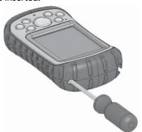
**Installing a CF or SD card.** To operate a card, insert the card into the appropriate card slot, located under the standard cap of the Field PC. (See the instructions in the previous section for removing the standard cap.) The system should automatically detect and use the card. However, if the card is not recognized, try the following:
