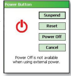
**Powering off the Field PC.** Powering off the device ends all programs and removes power from all system components except for the real-time clock. Unlike suspend mode, the device resets when it is powered on again.
