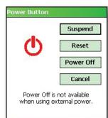
To power on the device, hold the power button until the green notification LED appears. The device is now booting. This process takes about a minute.
