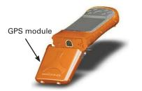
6. Align GPS module with the interface module.
