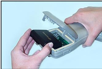
1. Push up on the release latches on the sides of the Allegro to open the battery compartment door.
