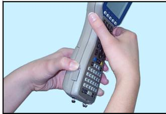
1. Push the battery door closed until each release latch clicks into place.
