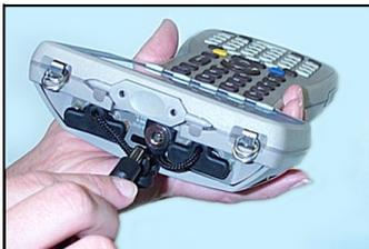
1. Remove the rubber protector from the Allegro's external power input jack.
