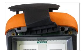
To install the new connector protector, insert the retention end into the area underneath the connector module. Press it underneath the battery door screw holes as shown.  When the retention end is installed correctly, it will look like the following photo. Make sure that the battery door gasket is seated in place along the edges as indicated.
