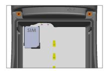
To remove the SIM card, pull the tray open and remove the card. Push the empty tray in until it catches.
