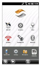
2. Tap-hold the Wi-Fi icon on the Home screen to go to the Wi-Fi control panel. When the handheld completes the scan, a list of available networks and their strenaths appears on the Wi-Fi Wireless screen.
