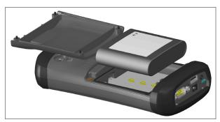
2. If you are using a micro SD card for additional memory or a SIM card with the 3G Data Modem (optional), you can install them now before you install the battery pack
