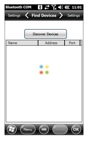
After the handheld searches, a list of discovered devices is shown. Select the device you want to connect to from the list and tap Connect. A COM port is automatically assigned for the device. You can change it to another COM port if desired. 3. The Archer 2 automatically tries to discover the PIN. You might be required to enter a PIN.
