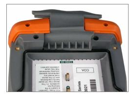
4. To install the new connector protector, insert the retention end into the area below the connector module. Press it under the battery door screw holes as shown.
