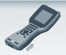
On both sides, slide latches up to open battery compartment door.
