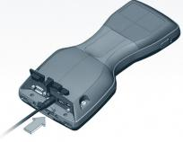
Plug battery charger into wall outlet, then into the Field PC. Follow on-screen instructions.
