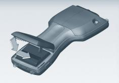
Place battery pack in the compartment and slide right.
