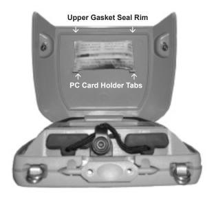
Note: If a piece of Velcro is already attached to the inside of the Allegro's PC card door, remove the piece on the new pack that has the removable adhesive cover and throw it away. Attach the desiccant pack to the piece of Velcro that is already attached to your Allegro.
